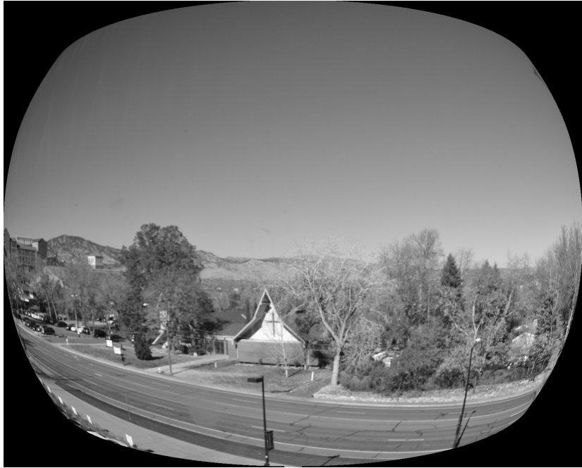
Figure 4.25: Barrel distortion under first order model used in the simulation at the extreme negative case: K_1 = -1.5 \times 10^{-8} .
