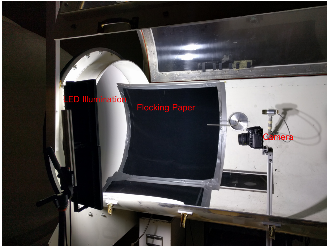
Figure 5.1: The image capture portion of the test setup. The flocking paper was used to reduce bright reflections off the tunnel walls.
